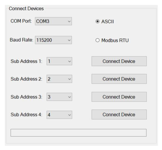
The current version of the "One Port Viewer" application supports the ASCII and Modbus RTU interface over serial COM ports communication.
