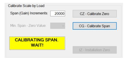
If the span calibration succeeded, the successful calibration will be indicated with a green message box in the left bottom of the "Calibrate Scale by Load" group box.
