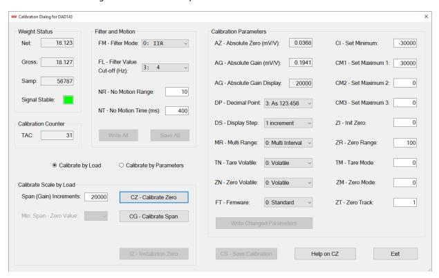
The "Calibration Dialog" consists of several sections covering different aspects of zero / span calibration.
