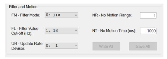
The value of the "No Motion Range" command can be increased to accept a wider range of motion increments when setting tare.
