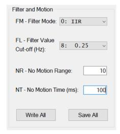
The value of the "No Motion Range" command can be increased to accept a wider range of scale instability (The range of accepted change of increments during the calibration measurement).
