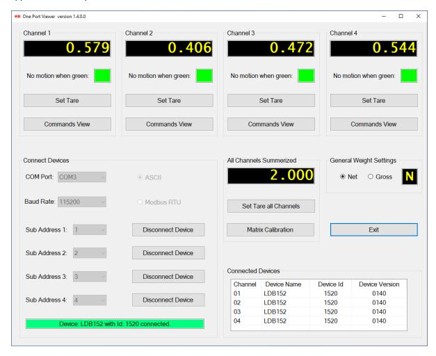
The main page consists of four channel groups from which load cell measurement and command settings can be performed. Calibration and tarring of H&B devices can be done from special "Calibration" and "Filter / Tare" dialogs found in the "Commands View" dialog, available for each of the up to four connected devices.
