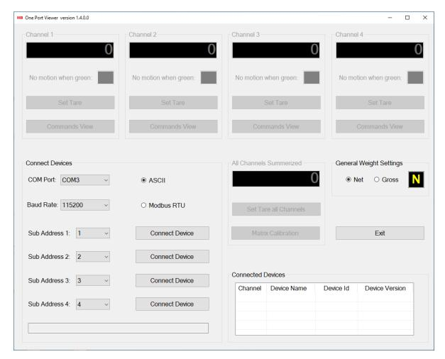
Start by defining the devices to be connected to the "One Port Viewer" application by configuring the settings in the "Connected Devices" group box.
