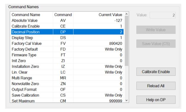
After the "Calibration Enable" command is sent, a given value of a writeable command in the calibration group can be changed and written to the device.
